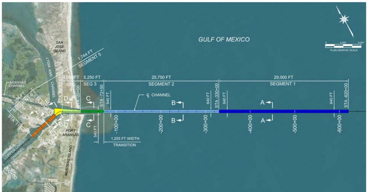
**Figure 1.1: Dredging plan for the Corpus Christi Ship Channel Deepening Project**
