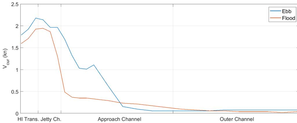
**Figure 4.3: Longitudinal Current speeds along the channel at the considered ebb and flood conditions**
