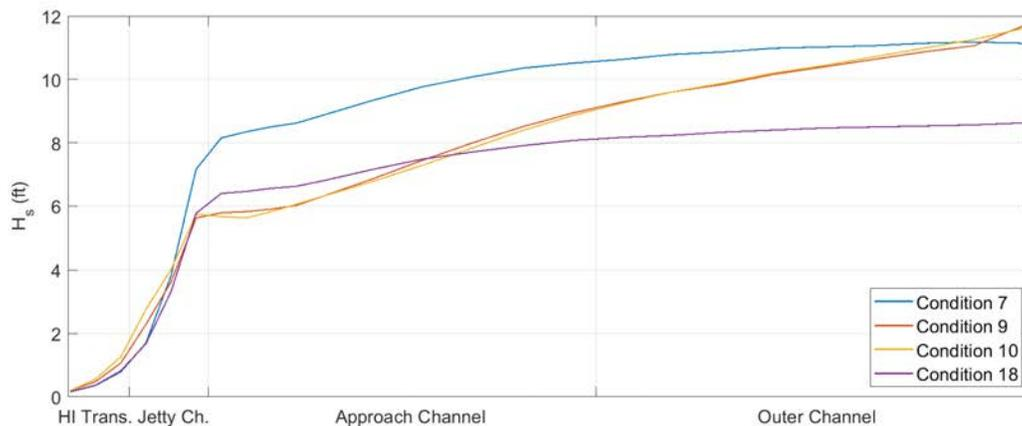
**Figure 4.5: Significant wave height along the channel for three extreme wave conditions (7, 9 and 10) and one operational wave condition (18)**
