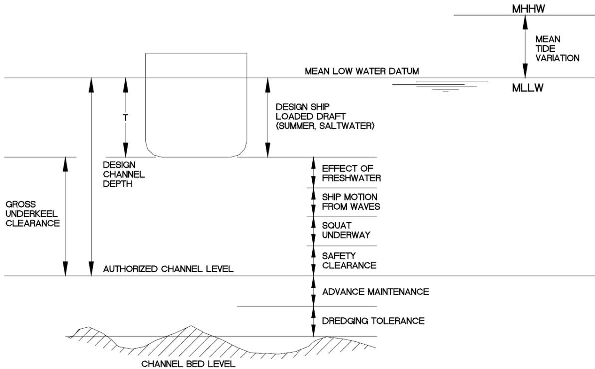
Figure 5.1: Channel depth allowances (source: USACE, 2006)
